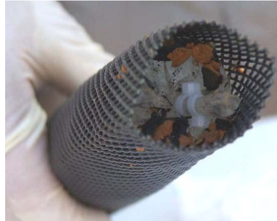
Figure 5-37. Top of RGC sampler showing deposits of large black and orange particles.
