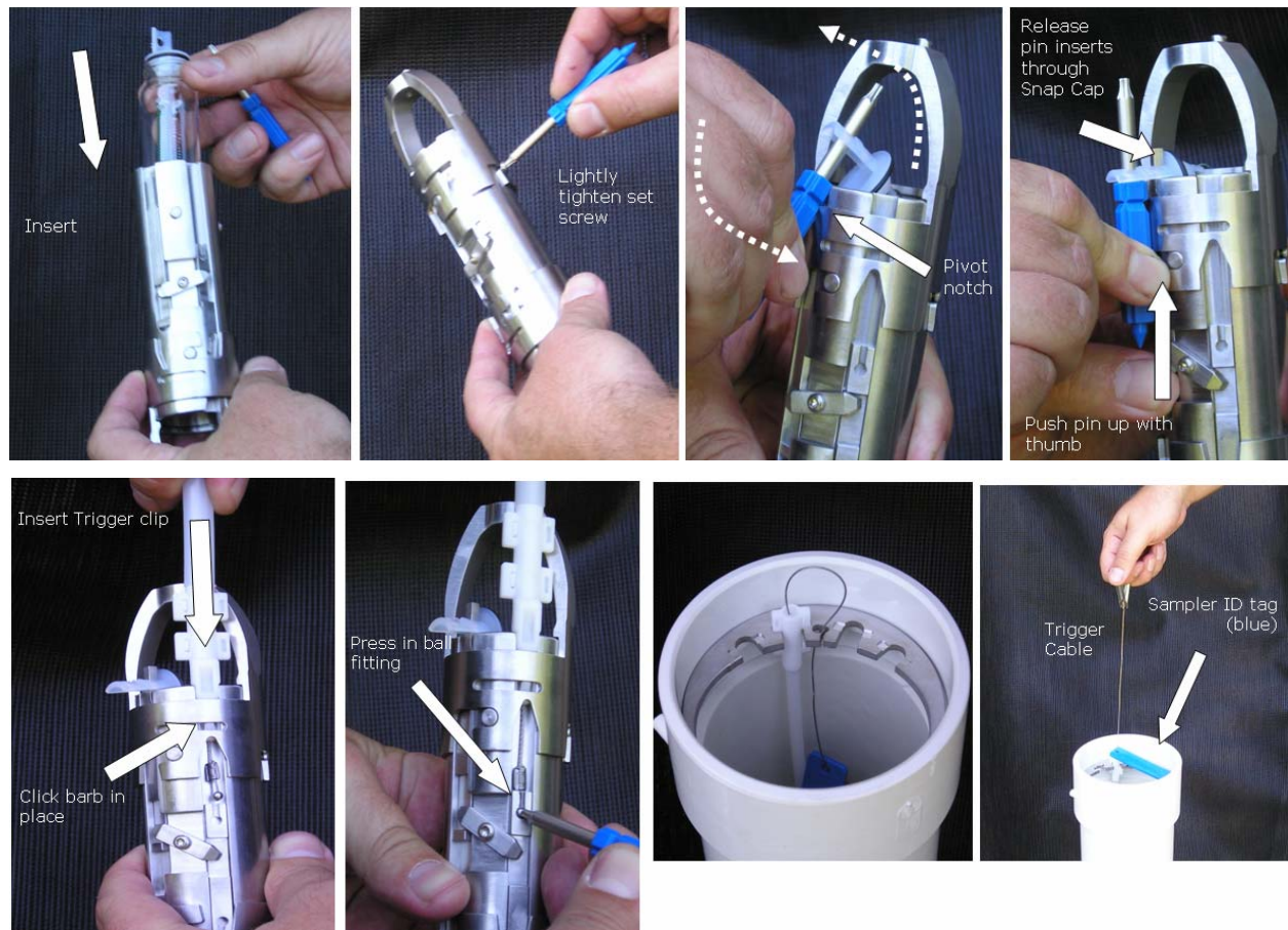
Figure C1. Snap Sampler deployment preparation.
